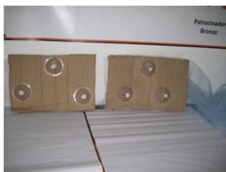
Demonstration of WHO cone tests on a bed net
